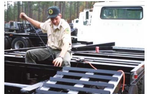
An employee runs wiring for the ramp on a transport.
