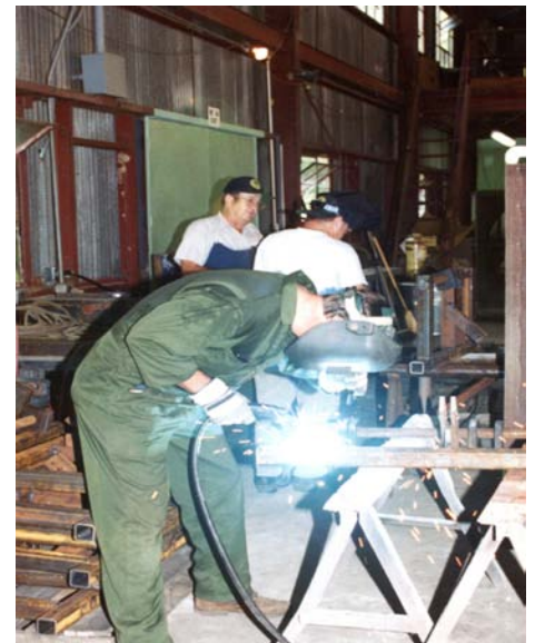
Welding experience was a big help in the fabrication of the truck bodies and beds.
